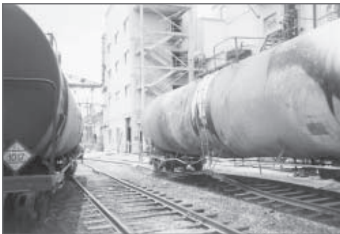
The seven-hour fire severely damaged the methyl mercaptan tank car (right) and a 90-ton liquid chlorine tank car (left). The intense heat also buckled the rail beneath the methyl mercaptan tank car.
