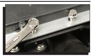
Figure 8 Tighten the Fuel Rail Bolts.
