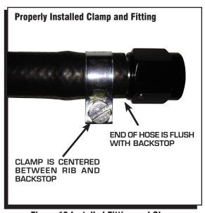
Figure 13 Installed Fitting and Clamp.
