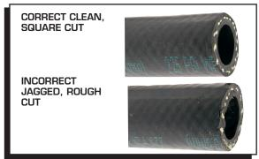
Figure 11 Severing the Hose Properly.
