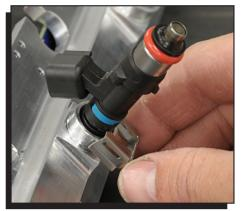
Figure 6 Installing the Injectors.
