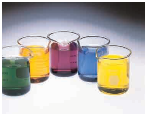
Various chromium compounds dissolved in water. From left to right: \text{CrCl}_2 , \text{K}_2\text{Cr}_2\text{O}_7 , \text{Cr}(\text{NO}_3)_3 , \text{CrCl}_3 , \text{K}_2\text{CrO}_4 .
