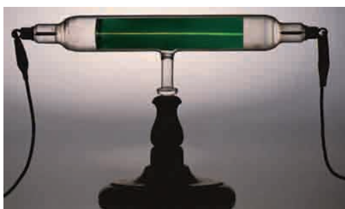
Figure 2.7 | A cathode-ray tube. The fast-moving electrons excite the gas in the tube, causing a glow between the electrodes. The green color in the photo is due to the response of the screen (coated with zinc sulfide) to the electron beam.
