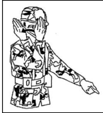
Figure A-5. Turn to right (starboard)
