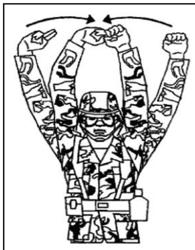
Figure A-23. Connect auxiliary power unit (day)
