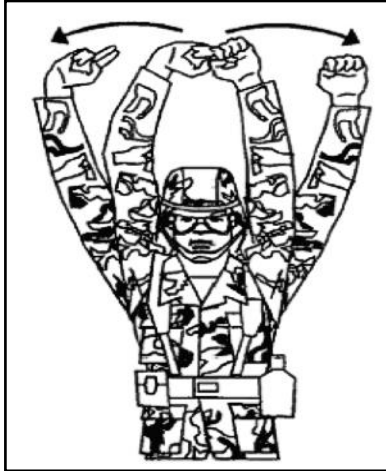
Figure A-24. Disconnect auxiliary power unit (day)
