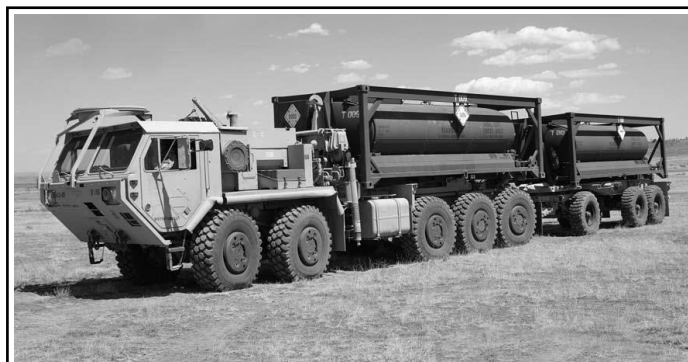
Figure 2-13. Modular fuel system with heavy expanded mobile tactical truck and trailer
