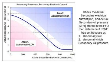
**TIP:** Consider performing the pressure testing using a mechanical pressure gauge **BEFORE** electrical testing and compare the test results (between the gauge and SM4 displayed values). Both test results should be very close. If there is a significant discrepancy between them (e.g. the (known good) gauge results are significantly higher than the SM4-supplied values), the pressure sensor would be suspect.
