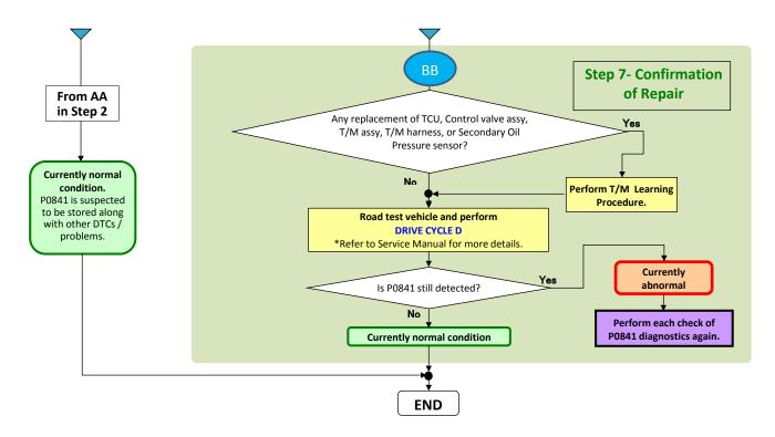
• In addition to the flow chart, use the following slides and information for additional help with accurately diagnosing a P0841:
