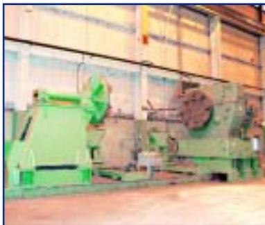
NILES FACING & TURNING LATHE
