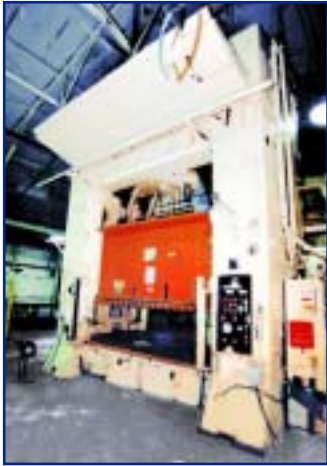
1 OF 4 400-T VERSON 4-POINT PRESSES
