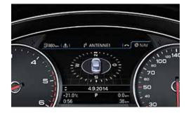
Driver information system with colour display\* shows the information of the driver information system on a high-resolution 17.78cm colour display with an even better overview and legibility; information from optional assistance systems and other MMI® system content can be displayed
