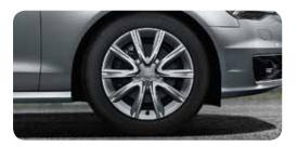
Cast aluminium wheels in 5-V-spoke design\* size 8 ] x 18 with 245/45 R 18 tyres
