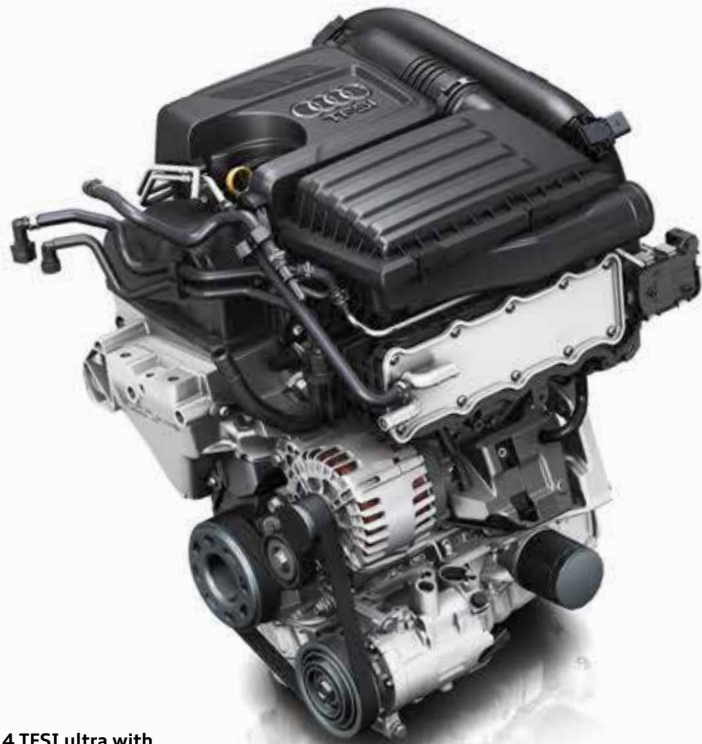
1.4 TFSI ultra with Audi cylinder on demand technology
