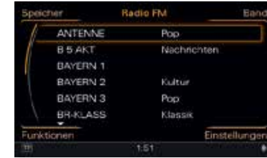
Radio: The integrated radio receiver is set up for VHF, LW and MW and optionally delivers digital radio with a continually updated station list
