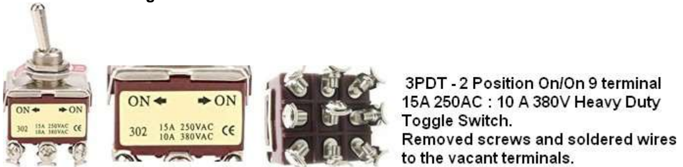
Fig 4. When switched to position (1) filter is Out, the battery is Off to the filter PCB and in position (2) filter is In and battery + supplied to the filter PCB...The 9 pin switch is wired the same as the 6 pin mini toggle switch (Fig 3) with the terminals 8 and 9 on the 9 pin heavy duty toggle switch being used to switch the battery + supply On/Off to the filter PCB. Terminal 7 not used.
