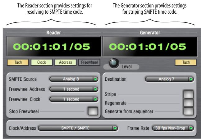
Figure 12-1: SMPTE Setup gives you access to your Audio Express's on-board SMPTE time code synchronization features.
