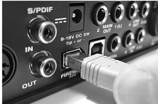
Figure 3-1: Connecting the Audio Express to the computer via FireWire.
