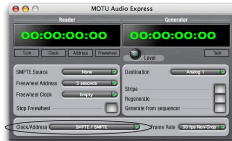
Launch the MOTU SMPTE Console to specify the time code frame rate and amount of freewheel. Also, confirm that the *Clock Source/Address* is *SMPTE/SMPTE*.
