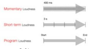
FIG 5. LOUDNESS ON THREE TIME-SCALES PER ITU-R BS.1770, BS.1771 AND EBU R128
