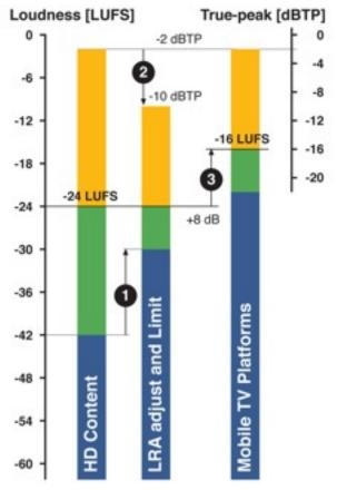
Fig 11. Automatic trickle-down from HD to Mobile and Pod Three easy steps when programs sit at -24 LUFS
