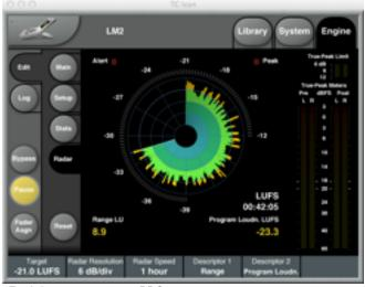
FIG 8. LOUDNESS PLOT OF BBC PODCAST THAT TRIGGERED THIS PAPER. PART OF THE PROGRAM IS TOO QUIET FOR AN IPOD
