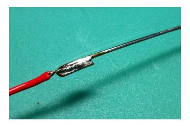
Next, I used 2 different diameters of heat shrink tubing to cover most of the length of the paper clip. This is to reduce the chances that it will contact other components by accident as I am probing around inside an enclosure, and to increase my ability to grip the probe since the paper clip by itself is pretty skinny and is fairly slippery. The heat shrink tubing may also provide some stress relief to the wire right at the solder joint by adding a little more stiffness.
