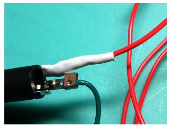
For some stress relief on the wires, I put a couple pieces of heat shrink tubing over both wires before screwing the female. Here's a picture of everything about to be screwed together:
