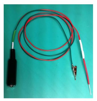
Obviously, this audio probe is designed to accept a guitar cable. You could also take an old guitar cable, cut off one end, and solder on a clip to the ground lead and the capacitor and probe to the hot signal carrying lead. Then you would plug the 1/4 inch male plug directly into your amp while testing.
