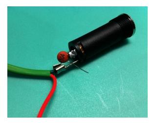
Then solder the probe wire to the other lead of the capacitor:
