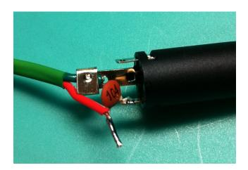
As I mentioned previously, I removed the green heat shrink. This was so I could take a larger diameter of heat shrink tubing, and use it to cover the solder joints of the capacitor. Here, I am about to slip the white heat shrink over solder joints and capacitor:
