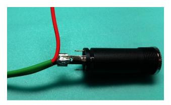
Next, solder one lead of the capacitor to the tip lug of the female audio jack as seen below:
