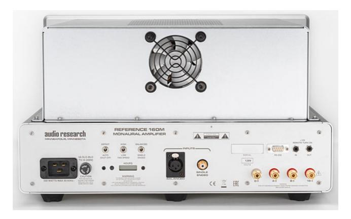
The cooling fan's speed is controlled with one of three small toggle switches on the 160M's rear. With the fan switched to High, I could hear it whirring in quiet musical passages; I stuck with Low. The only problem I encountered was that one fan didn't turn on—its connector cable had developed a kink. This kink master soon managed to bend the connection.
