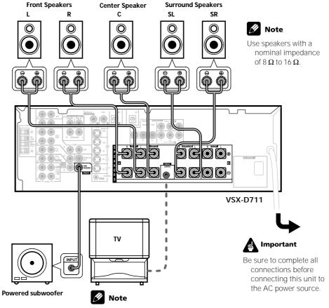
When using the speaker on your TV as the center speaker (C), connect the CENTER PREOUT jack on this unit to the audio input jack on your TV. In this case the center speaker shown is unnecessary.
