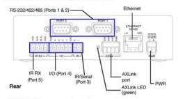
FIG. 2 NI-700 rear connectors and components
