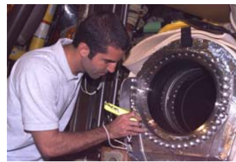
David Strait, Shuttle systems inspector with United Space Alliance, inspects a Space Shuttle Main Engine flow liner.
