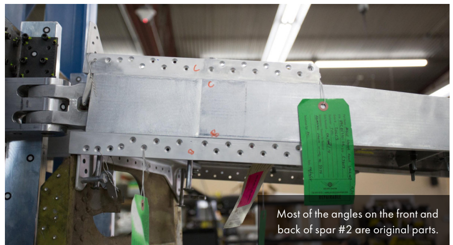
The "fitting assembly rib 26 3/4 and spar" is easier to see in this view.
