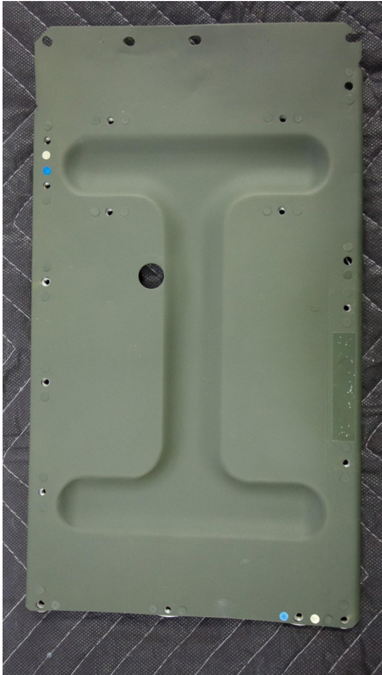
The original part after receiving an overall coat of color. On the center right side, a small rectangle of the original paint that has been left exposed in order to highlight the color match.
