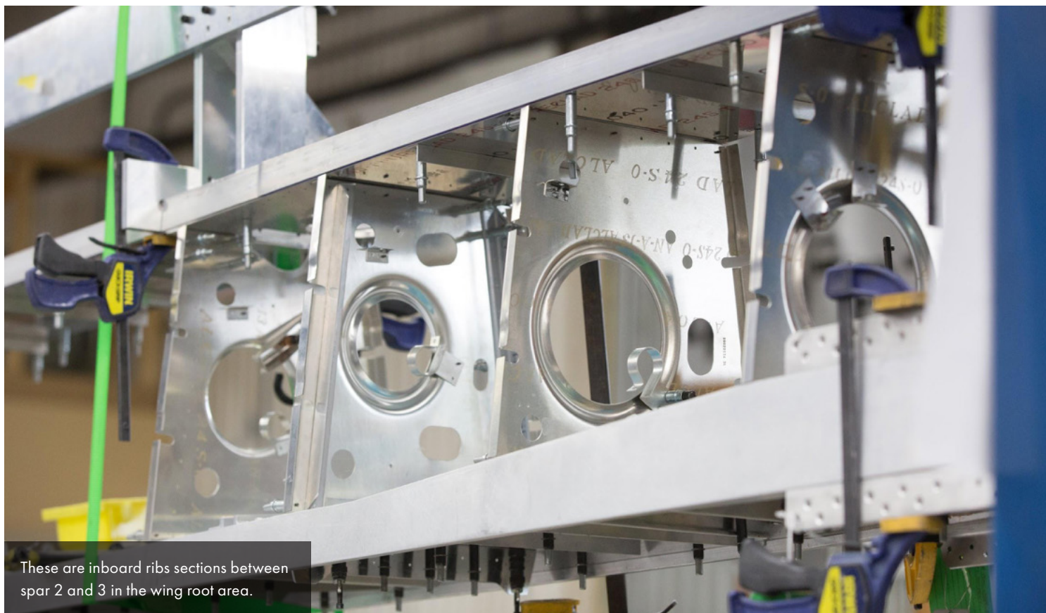
In this view, both inboard and outboard spar #3 sections show, as well as the straight continuous spar #2. The outboard wing rib sections between spar #2 and spar #3 are in place, along with some of the inboard ribs.
