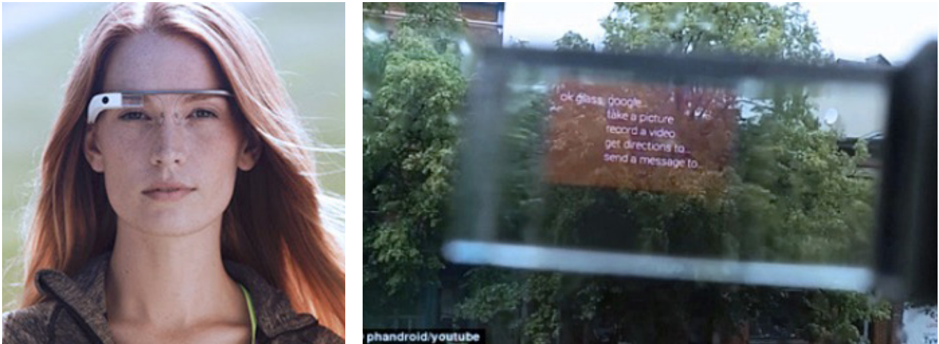
Google Glass, a heads-up augmented reality display.
