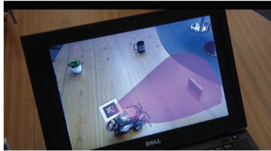
Figure 7. Augmented view on Lego Mindstorms robots. Sensor data is visualized as well as virtual objects are embedded into the real environment.
