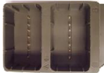
SPC adapter J-6878/P supports the AN/PRC-152 FALCON
