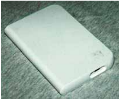
Figure 1. External 2.5-inch hard drive is about 0.6 inches thick and just under 5 inches long
