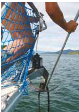
Pulling the last piece of heavy steel wire off the anchor
