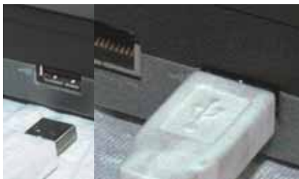
Figure 3. Standard USB connector at other end of cable shown plugged into the computer
