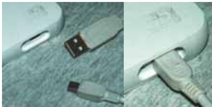
Figure 2. Disk mini-USB connection port, both ends of the USB cable and the mini-connector plugged into the port
