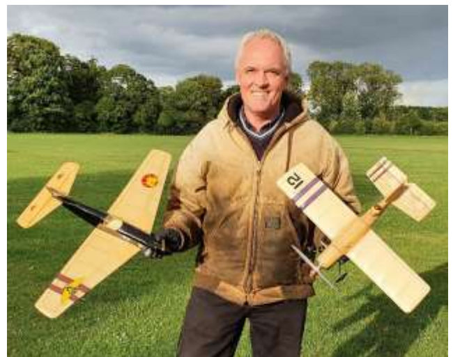
Tony with Peters KK Skystreak 26 with an Elfin 1.49cc on the left, and the Skyleada Hornet "A" class team racer with an ED Racer 2.49cc.
