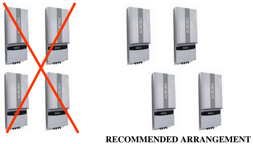
Fig.7 Recommended installation of AURORA inverters
