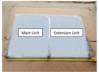
Connect the Main Unit with the Extension Unit and measure the distances between the Bracket mounting holes.
