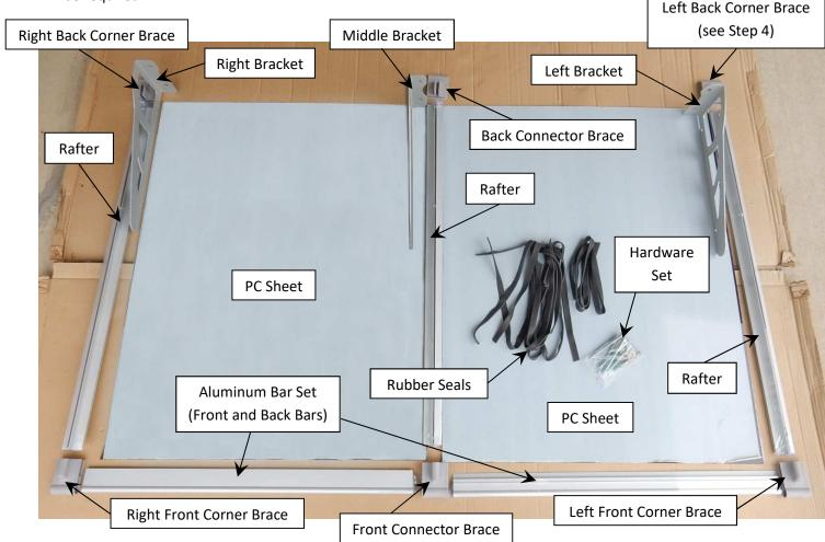
Arrange canopy parts to become acquainted with them. The above photo shows a canopy with 2 PC Sheets and 3 Brackets. Your canopy may have more or fewer PC Sheets and Brackets. Note that Bracket and Corner Brace names (left of right) are designated for viewing at the installed canopy from the outside in. The Middle Bracket can be either left or right. Corner Braces have slots to insert Aluminum Bars on only one side, Connector Braces have such slots on both sides.
