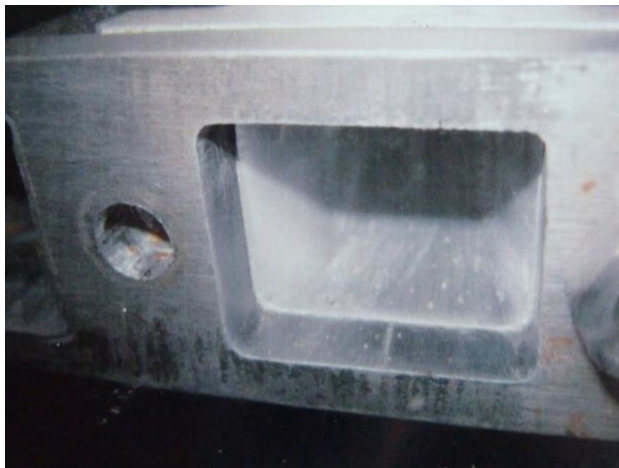
Smooth passage through manifolds
