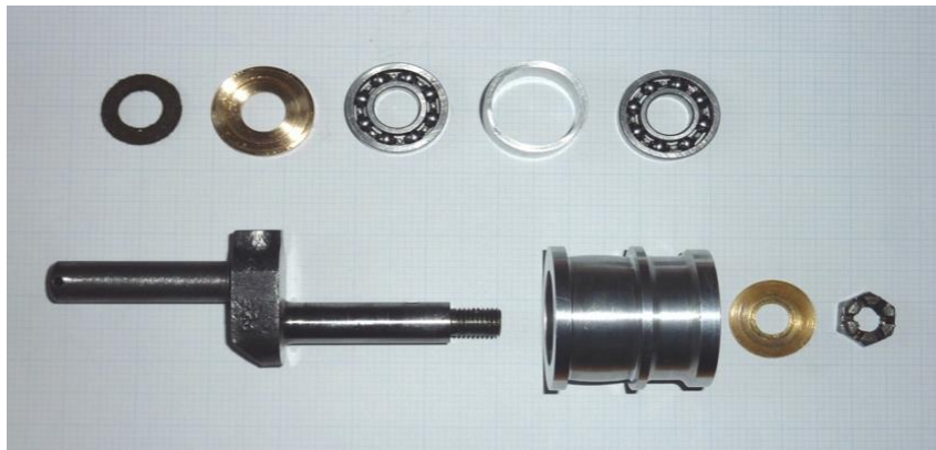
Spindle & components ready for assembly
