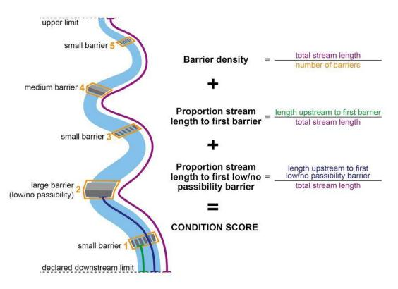
Figure 3. Diagram of the three fish barrier indicators and how they are calculated.
