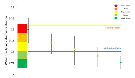
Figure 8. An example of how water quality grades are assigned. Where the middle point represents the annual median, the top whisker the 80th percentile and the bottom whisker the 20th percentile of the data. Only when the median meets or is better than the guideline (in this case meeting the guideline means the value must be at or below the guideline) can good or very good be scored. Scores for moderate, poor and very poor are equally scaled between the guideline and scaling factor.
