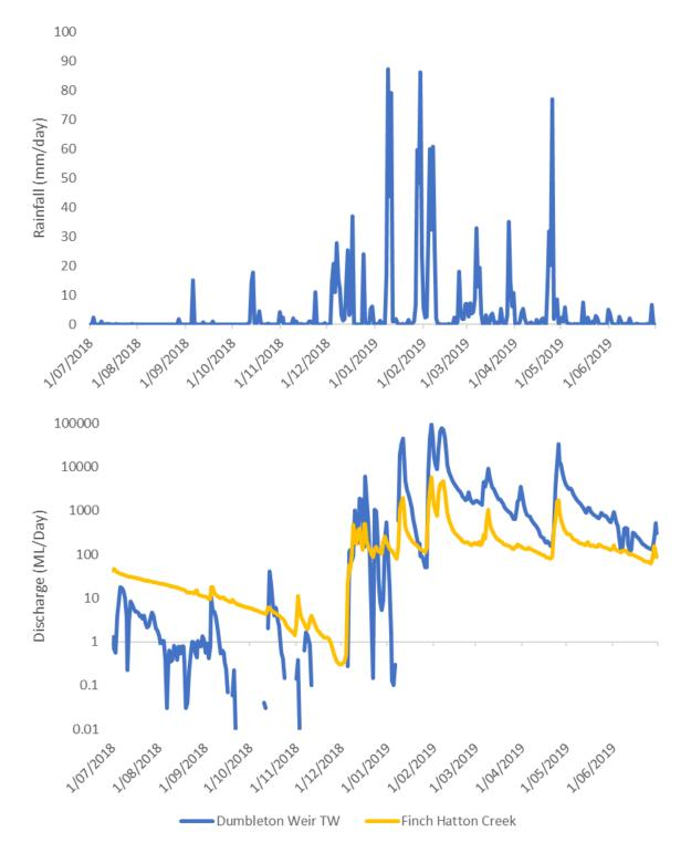
Figure 8. Rainfall for the Pioneer Basin and flow records for Dumbleton Weir Tailwater (TW) and Finch Hatton Creek for 2018-19. Flow (ML/day) is represented in log scale.
