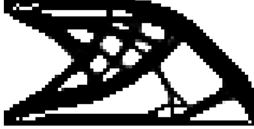
Figure 3: Tip cantilever beam with length scale control.
