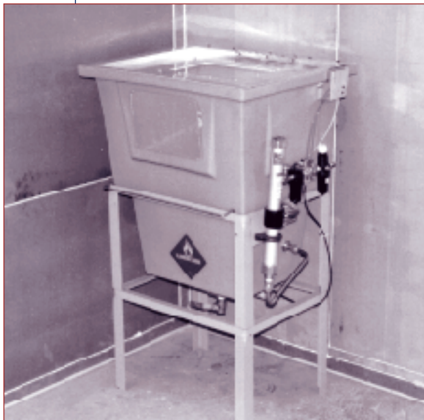
Figure 12: Enclosed Air Powered Mechanical Cleaning System
