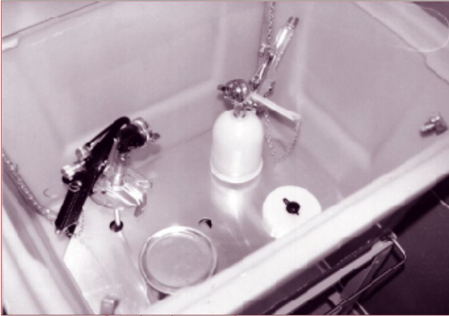
Figure 13: A Two Gun Capacity Gun Wash System
