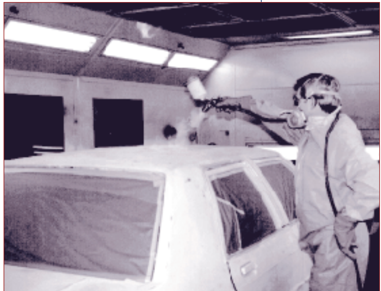
Figure 17: Application of the Primer-Sealer
