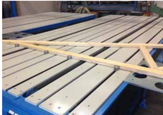
Robust pucktable with precise positioning and fast set up. Add an extra puck per slot as an option to enable double amount of support compared to traditional system.
