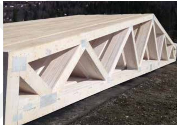
Each nail plate is placed exactly right relative to the joint. The press visually identifies each joint and position the nail plate exactly even if the truss has a deviation in length or shape.
