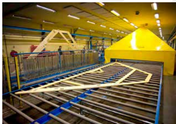
The press picks, positions, places and presses the nail plates automatically.
