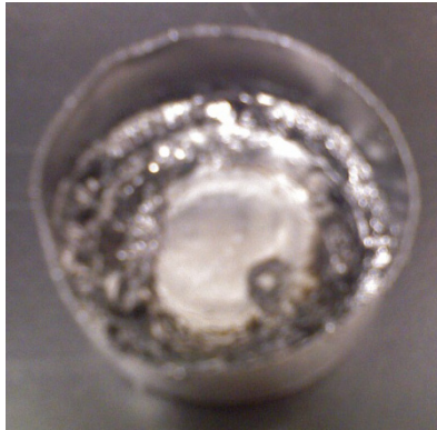
Figure 9. Olive oil pan after no ignition occurred.
