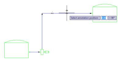
A leader line is automatically placed to connect the annotation bubble to the control valve.
