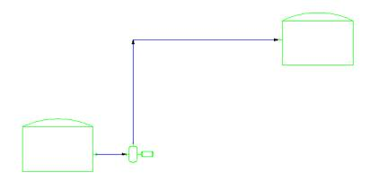
**Note** To view a flow-direction error, start the schematic line at the pump and end it at the tank. You can then reverse the flow to fix the error. To reverse the flow, click the line and on the ribbon Home tab ➤ Schematic Line panel, click Edit. In the list, click Reverseflow. Press Enter.
