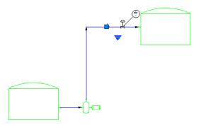
**2** Drag the gate valve from the horizontal line, and click on the vertical line to place the valve.
