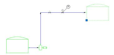
**2** On the lower-left corner of the selected tank, click the grip and drag the tank to the left, about half the length of the horizontal line. Click again to place the tank in the new position.
