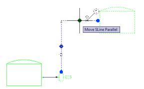
**2** Click the stretch grip in the middle of the top horizontal line, and move the line up slightly. Click the new location to place the line.
