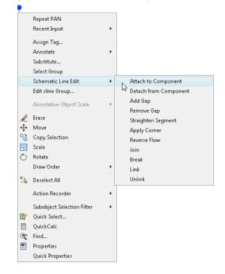
quick access to tasks such as assigning a tag, annotating the line, substituting a line type, and various options for schematic line editing.
