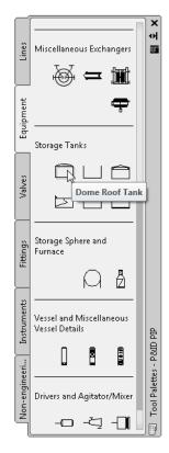
2 Click any open area in the upper-right section of the drawing area to specify a location for the tank.
