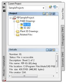
The Project Manager also provides access to the Project Setup dialog box, which is used by administrators to configure the drawing environment based on your company or client requirements.
