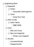
By creating a customized Data Manager view, you can view drawing data with the focus on properties instead of classes. For example, you can set up existing properties, such as Manufacturer and Supplier, as the basis of the new view. You can also create and use new properties for a view.
