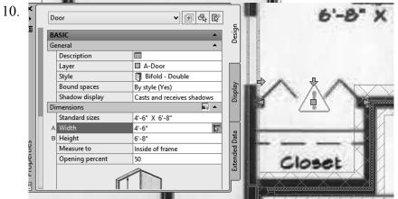
Place the **Bifold - Double** door at the closet next to the entry way.
