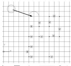
Let's move the small circle so it is concentric to the arc using a geometric constraint.
