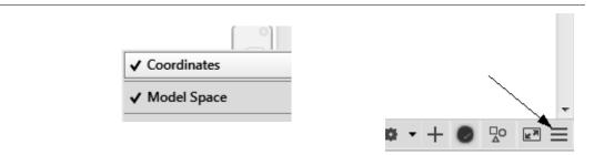
To toggle the display of coordinates, left click on the Customize tool in the lower left of the screen and left click on Coordinates in the list.
