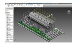
Align Equipment and Skids with Piping Design. With the equipment and skid design features of Autodesk Plant Design Suite, you can import 3D models from Autodesk Inventor into AutoCAD Plant 3D and intelligently connect to the piping. There is no need to remodel the equipment and skids.
