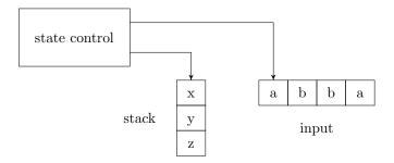
In addition to the finite automaton-like structure it has, it also has a stack on which which symbols can be written down and read back later (The concept of a stack is hopefully familiar to the reader). This stack, which has infinite memory, is what enables the pushdown automaton to recognize languages such as  $\{0^n1^n \mid n \ge 0\}$  because it can store the number of 0s it has seen on the stack. The "pushdown" in pushdown automaton corresponds to the stack structure.
