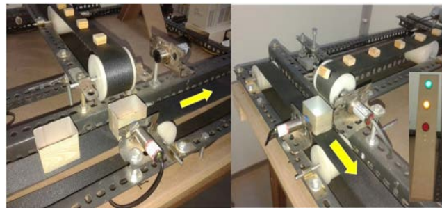
Fig. 21 Inductive Sensor Activated as the box be in location.
