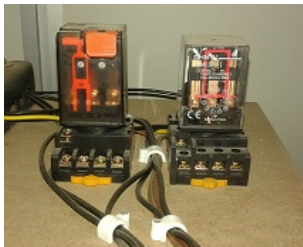
Fig. 10 Relay's Setup on the Project.
