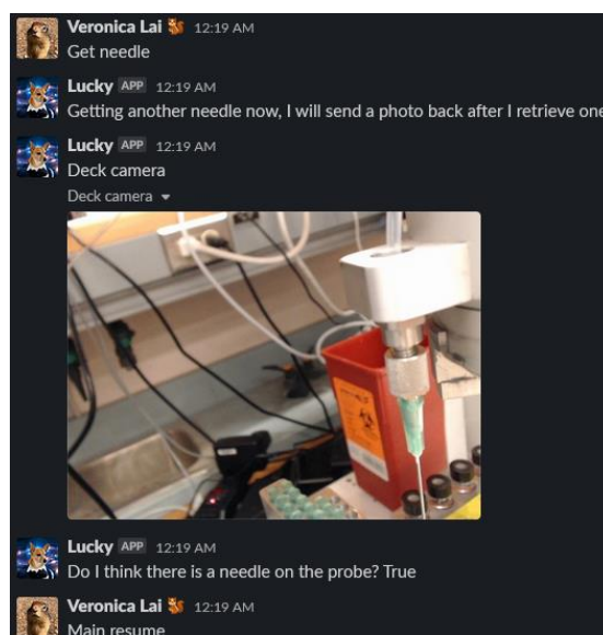
Fig. S10. Needle cap and uncapping control with vision: (A), after unsuccessfully getting and uncapping a needle, a message was sent by the Slack app detailing the issue and prompting the researcher to take control to remedy the issue. (B), a command to uncap the needle was sent but it looks like there is an issue with trying to uncap the needle, most likely the cap was on too tight. (C), the command to remove the needle is sent and was executed successfully. (D), the command to get and uncap a needle was sent and was executed successfully, and the command to resume the experiment was sent.
