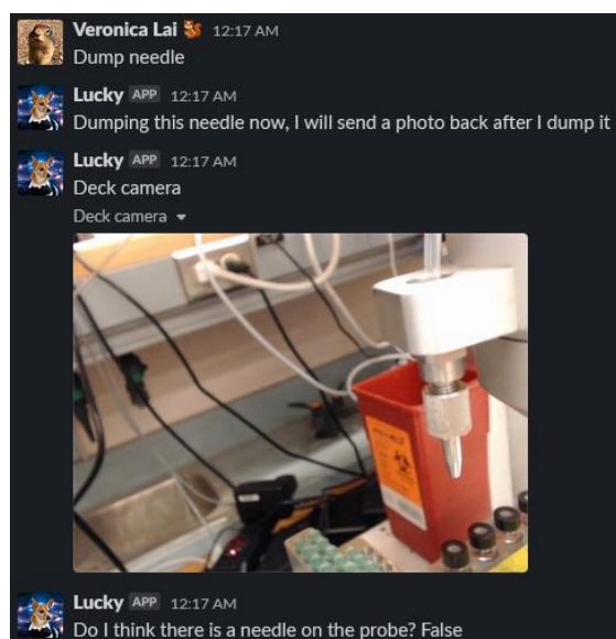
Fig. S10. Needle cap and uncapping control with vision: (A), after unsuccessfully getting and uncapping a needle, a message was sent by the Slack app detailing the issue and prompting the researcher to take control to remedy the issue. (B), a command to uncap the needle was sent but it looks like there is an issue with trying to uncap the needle, most likely the cap was on too tight. (C), the command to remove the needle is sent and was executed successfully. (D), the command to get and uncap a needle was sent and was executed successfully, and the command to resume the experiment was sent.
