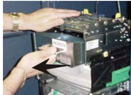
Removing the reject vault
