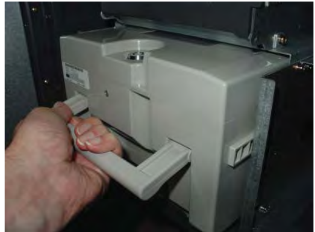
Removing note tray from the dispensing mechanism.
