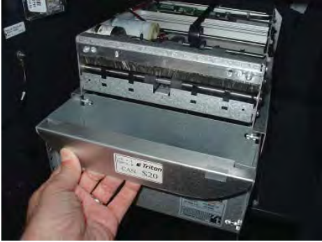
Removing note tray from the dispensing mechanism.
