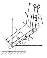
• Use Lagrangean equations to determine the dynamic equations of the robot
