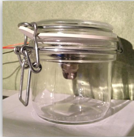
Figure 18: The glass pot which used to adjust the MQ-2 sensor
