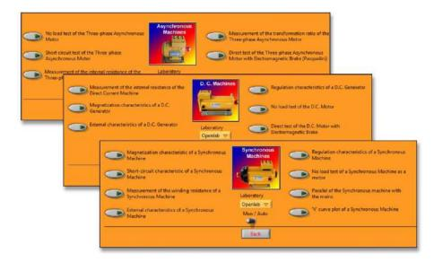
The **DL 8330SW** is a software developed for the acquisition and display the data of the DL OPENLAB\_A laboratory. It is developed in LabVIEW and communicates with the instruments (DL 10065N and DL 10050N) through the data acquisition module (DL 1893) and collect mechanical data (speed and torque) as well as electrical data (AC and DC, Voltage, current and Power).
