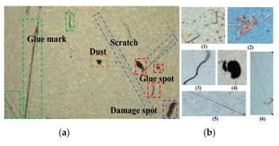
Figure 1. Challenges of detecting surface defects of metallic components. (a) Defects with various shapes and sizes, (b1) defects with ambiguous edges and low contrast, (b2) defects with different background, (b3) fiber, (b4) dust, (b5,b6) scratches.
