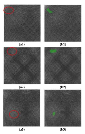
**Figure 9.** Examples of CASAE-processed images with textured backgrounds. The first columns are examples of (**a1–a3**) defects images and (**b1–b3**) result images of defects marked in green.
