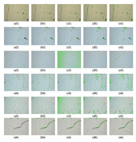
**Figure 6.** Segmentation results. The six rows are examples of defective images. (**a1–a6**) raw images, (**b1–b6**) results of Kittler [19], (**c1–c6**) results of Otsu [17], (**d1–d6**) results of a fully convolutional network (FCN) [36], (**e1–e6**) results of the cascaded autoencoder (CASAE) (proposed).
