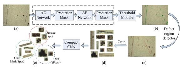
**Figure 2.** The pipeline of the proposed metallic surface defect inspection architecture. (**a**) Original image, (**b**) defect segment, (**c**) defect location, (**d**) cropped results, and (**e**) classification.
