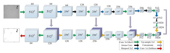
Figure 3. The architecture of the autoencoder (AE) network.
