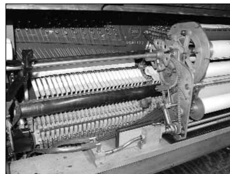
The piano action and left side of roll changer.
