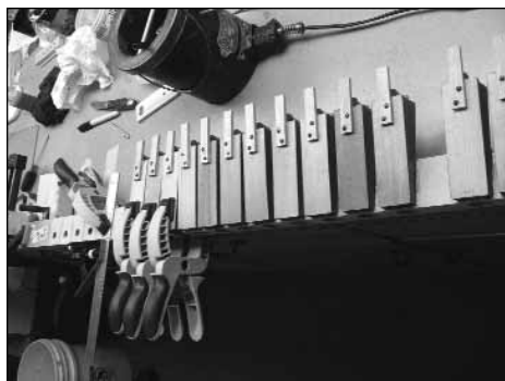
Recovered pneumatics being glued to one deck.
