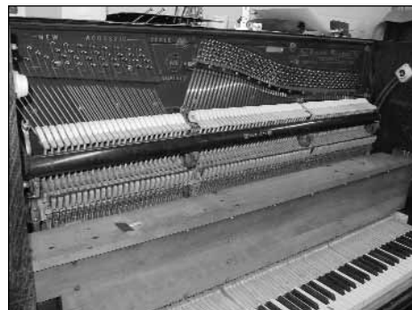
New hammers installed, action regulated and stack being installed.
