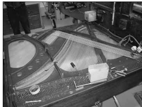
Restringing in progress.
