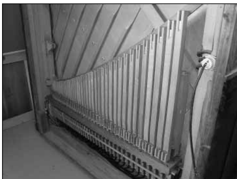
The pipe chest and two ranks of pipes installed inside back. The violins show, with the stopped flutes hiding between them and the soundboard. The massive piano cabinet and plate provide support for the string tension without the usual back posts.
