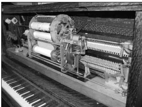
Automatic music roll changer and other parts installed above keyboard.
