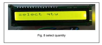
Fig 7 Shows the validation process in which after the card is flashed, RFID Reader will access its unique 12 bit HEX Code. It will compare the ID with stored database. Fig 8 shows about the selection of quantity, after the validation is done the amount of quantity is been selected by user using the keypad.
