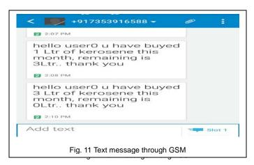
Fig 11 Shows the Text message through GSM, which includes the details about the quantity of kerosene purchased by the user and the remaining quantity from the user monthly quota, has sent to the registered mobile number of the user through the GSM via SMS.
