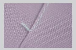
Clean-cut at end of the seam (< 5mm)
