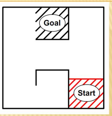
Basic – Start motor at 63 for 2 seconds, Stop motor, start motor, point turn left, stop motor...
