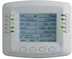
Indoor Control Panel
