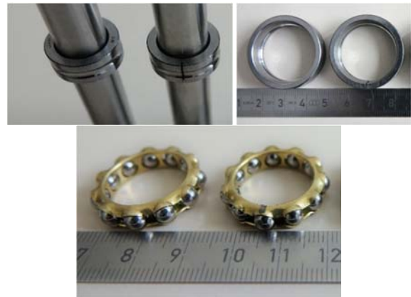
Fig. 3. Artificially damaged bearings, each w/o damage (left) and small damage (right); Inner ring damage, outer ring damage, and rolling element damage.
