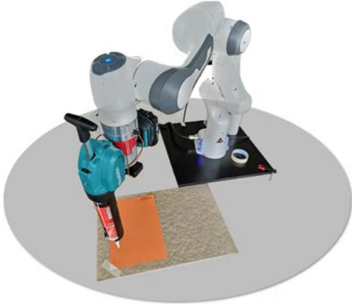
Fig. 1. Experimental setup: Franka Emika Panda robot with a Makita caulking gun connected through a custom flange.
