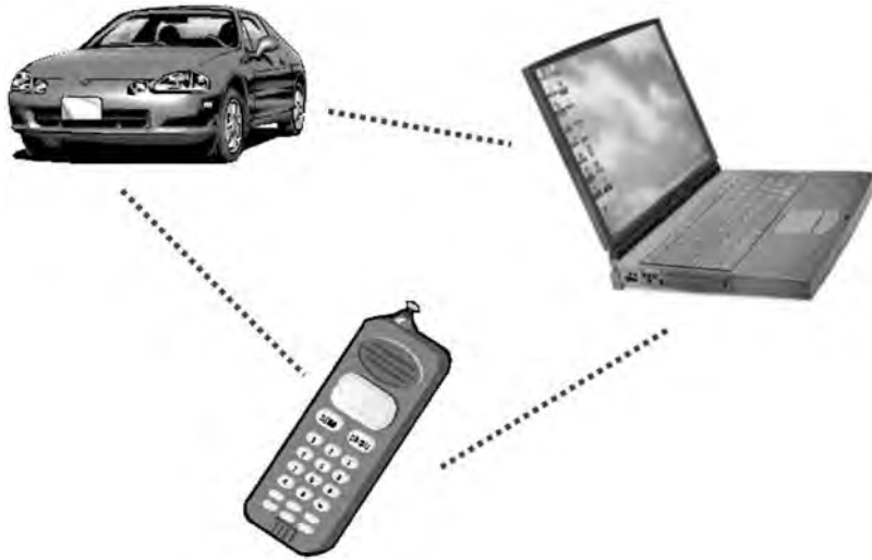
Figure 4.34 Representation of a Bluetooth network – a piconet
