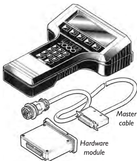
Figure 3.20 Lucas Laser 2000 Tester
