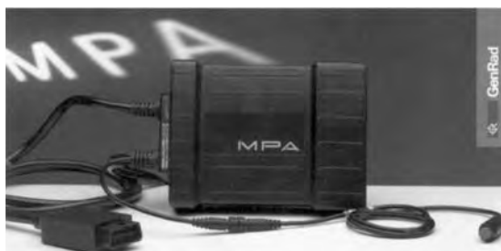
Figure 3.25 Multi protocol adapter
