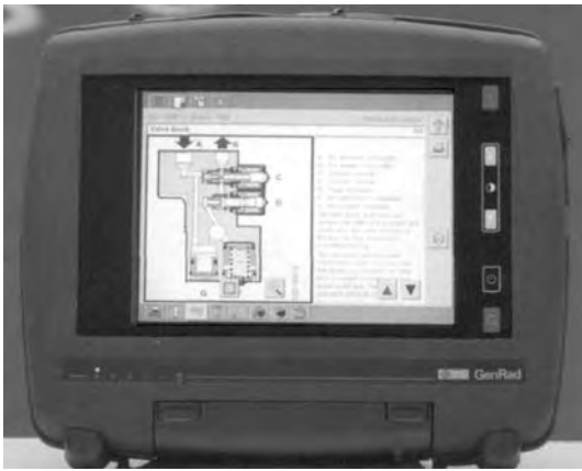
Figure 3.24 GenRad diagnostic system
