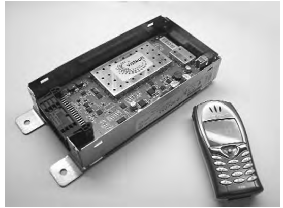
Figure 4.35 Visteon's Bluetooth Interface Module (Source: Visteon)
