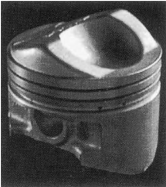
Figure 10.27 Optimum piston shape
