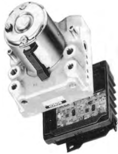
Figure 15.8 ABS and traction control ECU on the modulator
