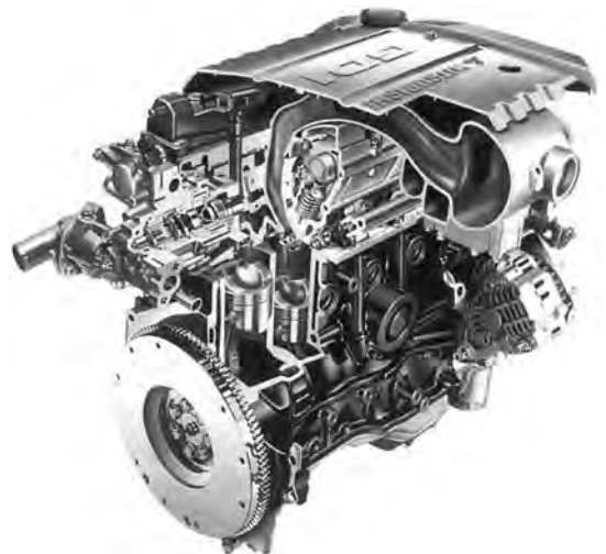
Figure 10.23 Mitsubishi gasoline direct injection 'GDI' engine
