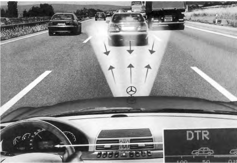
Figure 16.14 Adaptive cruise control operation
