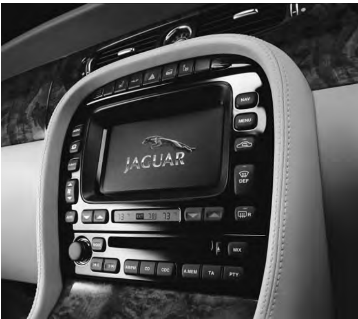
Figure 13.36 Jaguar DVD/Navigation touch screen (Source: Ford)
