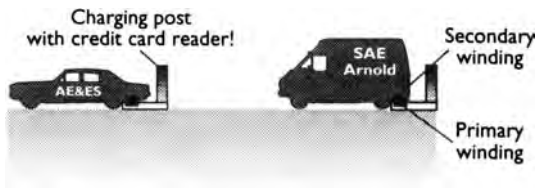
Figure 17.13 Inductive charging could help the development of the electric vehicle
