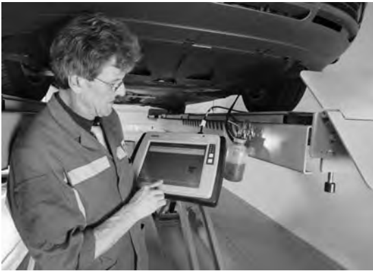
Figure 3.42 Diagnostic tester in use for bleeding a brake system (Source: Bosch Press)
