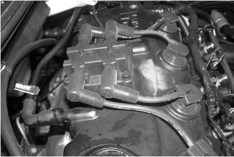
Figure 8.41 Distributorless ignition coil in position
