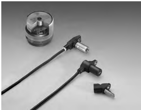
Figure 15.28 Progress in ABS wheel speed sensors (Source: Bosch Press). The ABS wheel speed sensors have become increasingly smaller and more efficient in the course of time. Recent models not only measure the speed and direction of rotation but can be integrated into the wheel bearing as well
