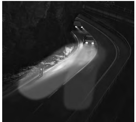
Figure 11.30 Situation where AFS improves target detection (Source: Visteon)
