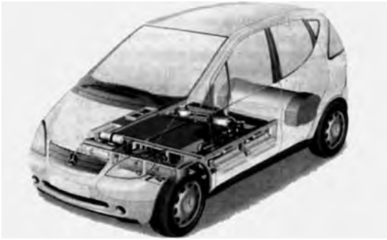
Figure 5.13 NECAR – Fuel cells in a Mercedes A-class
