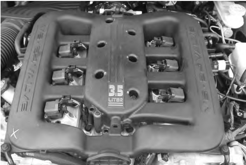
Figure 8.42 Six direct ignition coils in position. Some systems use CDI
