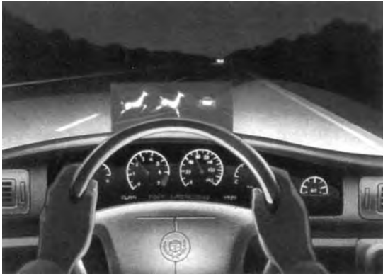
Figure 11.24 Night vision system in use
