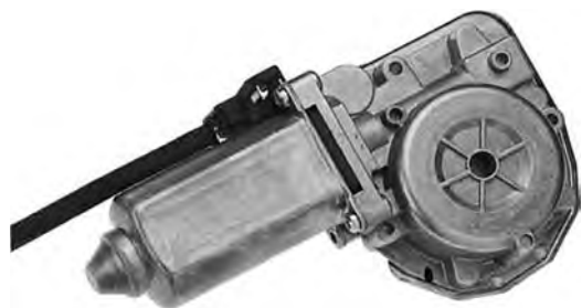
Figure 16.11 Window lift motor for cable or arm-lift systems
