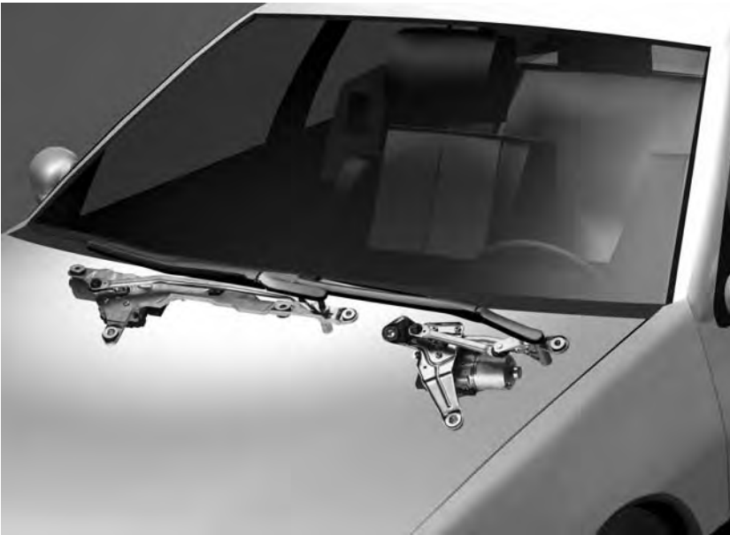
Figure 12.23 Twin-motor wipers in position (Source: Bosch Press)
