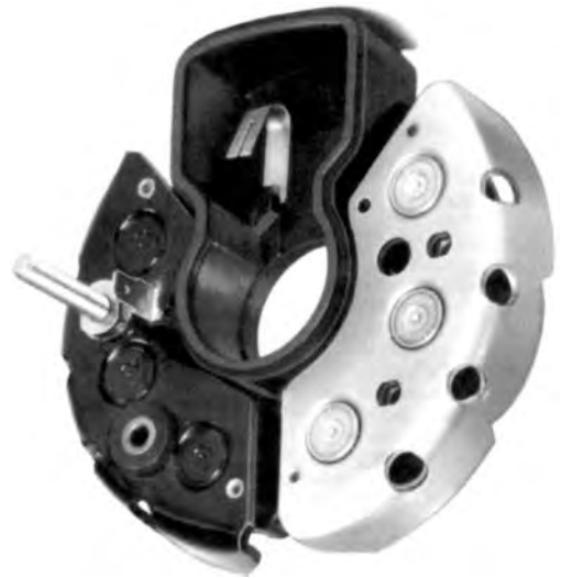
Figure 6.12 Rectifier packs in common use
