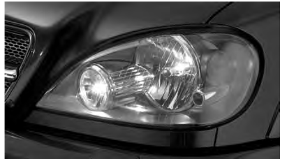
Figure 11.33 Xenon lighting (Source: Visteon)
