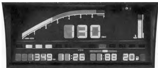
Figure 13.16 A display using LEDs
