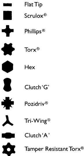
Figure 3.2 Many types of 'driver' shapes are now in use
