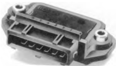
Figure 8.15 Transistorized ignition module
