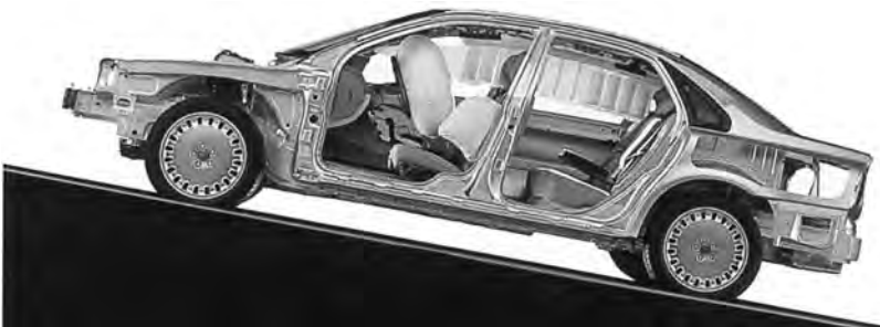
Figure 16.42 Volvo S80 airbags
