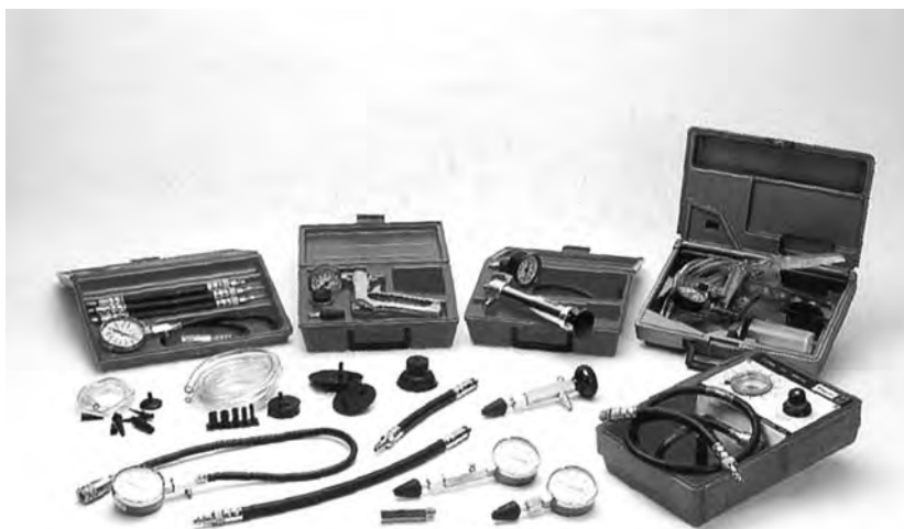
Figure 3.14 Pressure testing equipment
