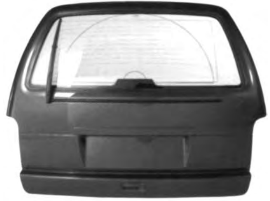
Figure 12.20 Linear wiper system
