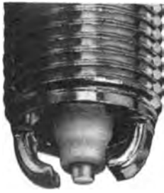
Figure 8.30 The semi-surface spark plug has good anti-fouling characteristics
