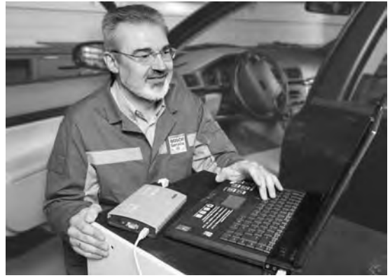
Figure 3.43 Taking a readout from the control unit memory (Source: Bosch Press)
