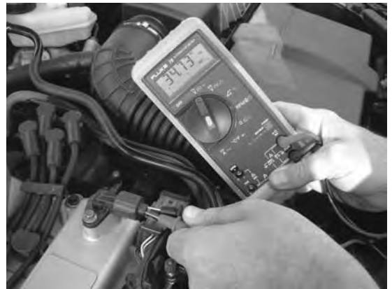
Figure 3.5 Crankshaft/Camshaft sensor test
