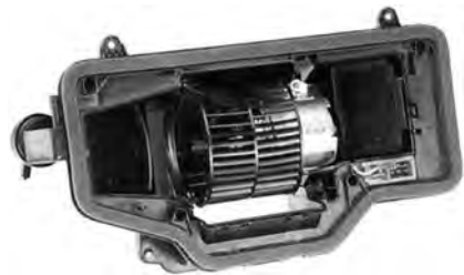
Figure 14.4 HVAC motor mounted in spiral housing
