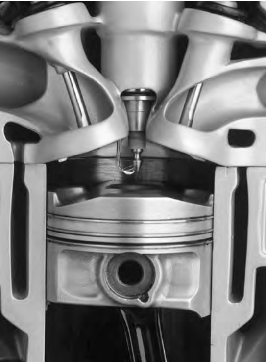
Figure 10.69 Combustion control spark plug injector (Source: Saab)
