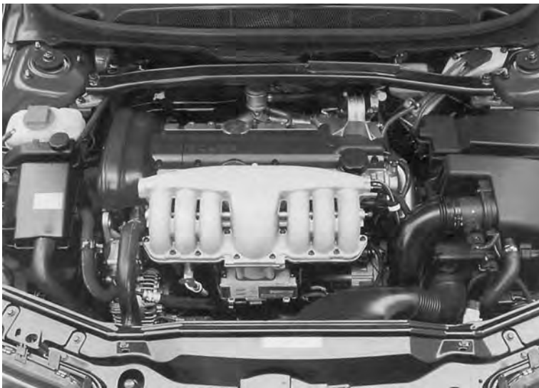
Figure 10.4 Volvo engine showing the feature of the inlet manifold design
