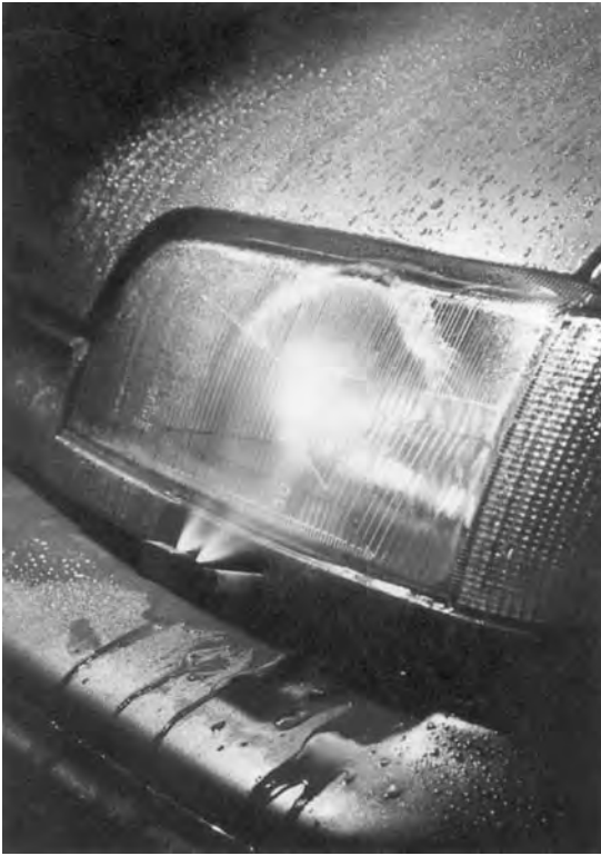
Figure 12.15 Headlight washers in action
