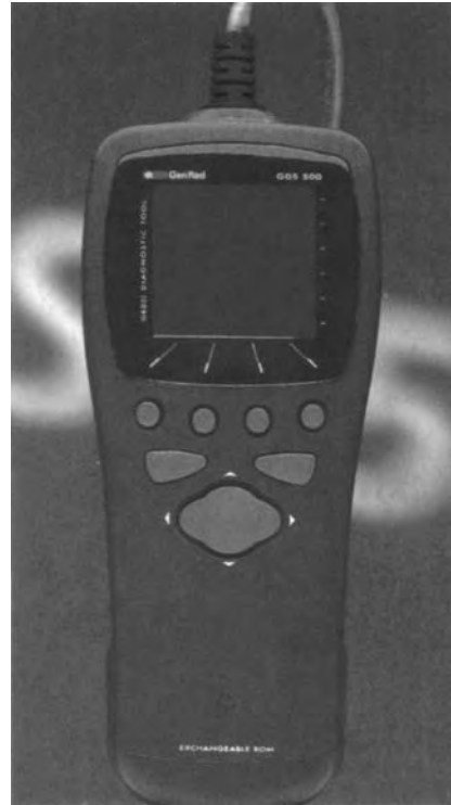
Figure 3.17 OBD II scanner
