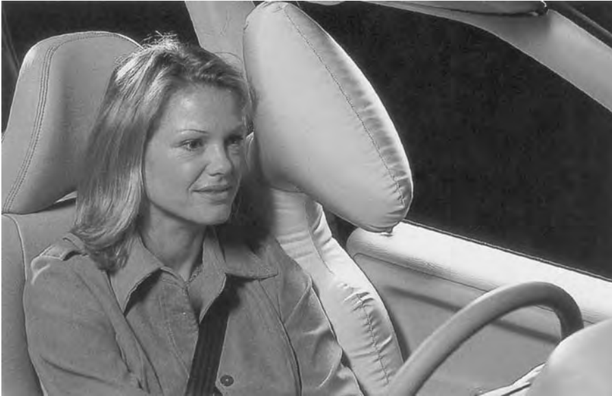
Figure 16.44 Volvo new SIPS airbag
