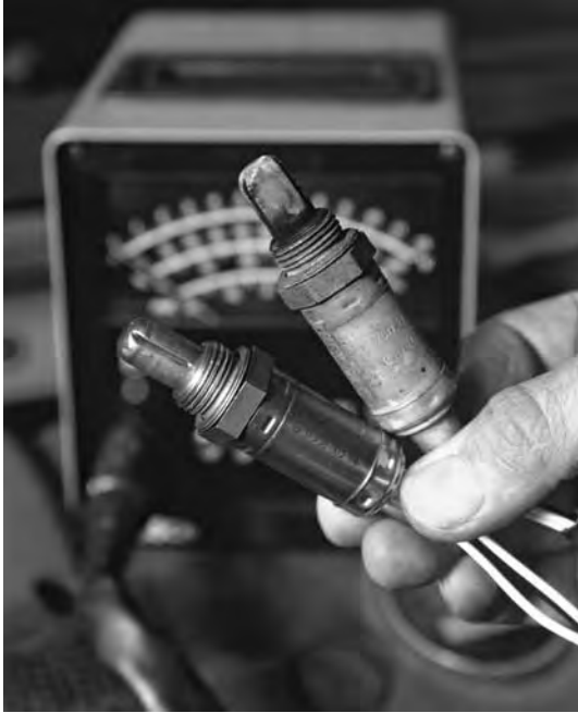
Figure 2.86 Lambda sensor's performance should be tested (Source: Bosch Press)
